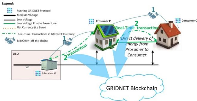
Figure 6: Bids and offers happen off the chain, while finalizations of transactions are included inside of it.
