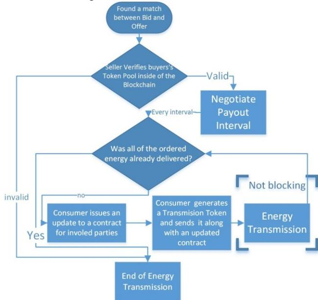
Figure 4: Energy transaction and transmission process.
