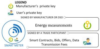
Figure 3: Energy measurements are signed by a DSO's or manufacturer's private key while everything else is signed by the user.
